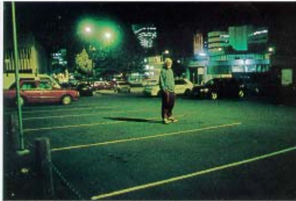
Figure 7. This shows what not to do in a carpark, with strong shadows from the single-direction lighting. The new standard requires lighting from two, opposed directions.
