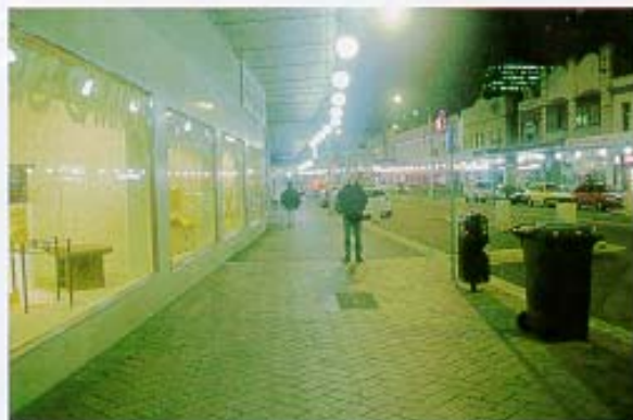
Figure 1. A footpath beside a traffic route with supplementary under-awning lighting.
