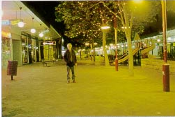
Figure 4. A pedestrian mall lit to P1 standard with a high vertical illuminance.
